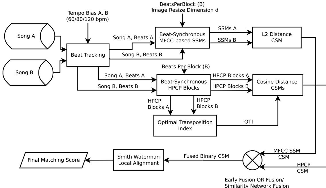
FIGURE 3.11: A block diagram of our extended system which performs early fusion of MFCC SSMs and HPCP before scoring with Smith Waterman. This pipeline is the same for OR fusion and similarity network fusion before the fusion happens.
