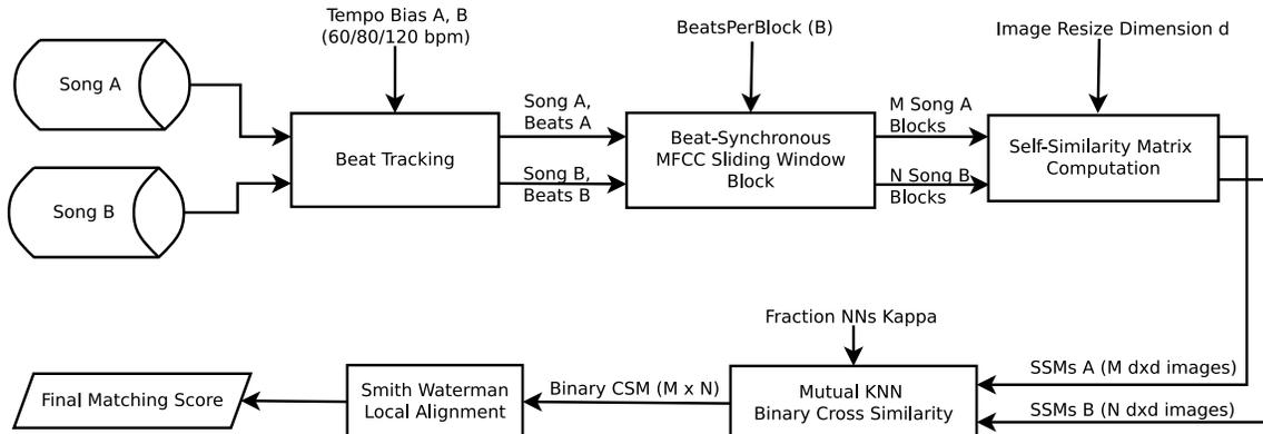
FIGURE 3.7: A block diagram of our system for computing a cover song similarity score of two songs using MFCC SSMs.
