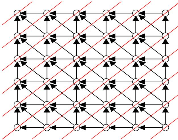
FIGURE 5.6: A schematic of the linear systolic array used to compute DTW in parallel. Elements of the dynamic programming matrix are drawn as circles. Black arrows are drawn to show dependencies between elements in the dynamic programming matrix, and red arrows show elements which can be computed in parallel if the processing occurs from the upper left  $(0, 0)$  to the lower right  $(M, N)$ .
